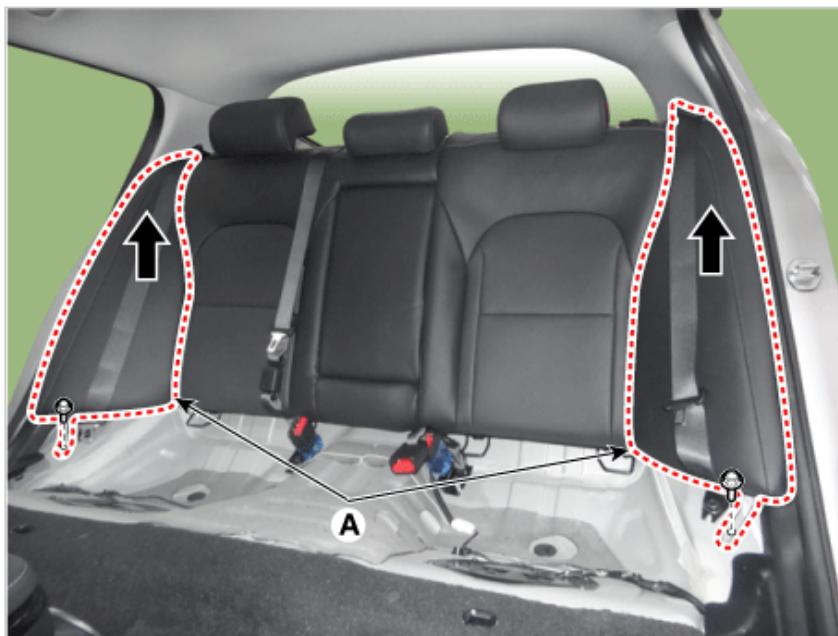
4. Disconnect the rear center seat belt (A) after pressing the groove in the direction of the arrow.
