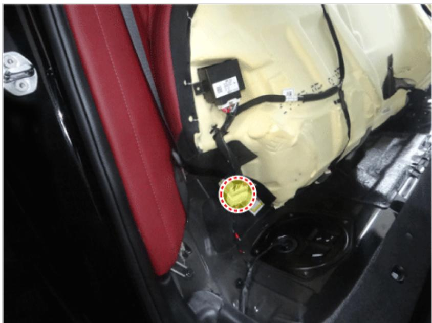
3. Remove the rear back side seat (A) by pulling it up after loosening the mounting bolts.
