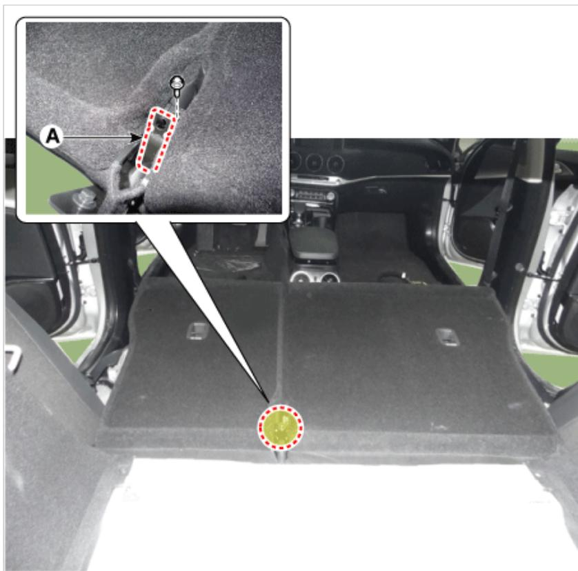
7. Remove the rear seat back assembly (A).
